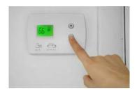
Make sure switch is <u>firmly</u> in the heat position Turn off and back on to reset the system If digital look for low battery indicator - change batteries if old
